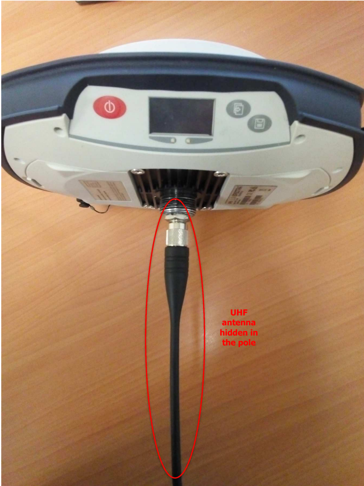
UHF antenna without the pole
