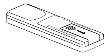
B: Insert 2 AAA batteries according to the markings inside compartment
