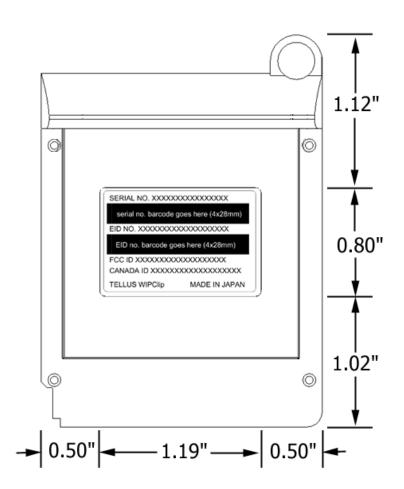
Figure 1 - WIPclip V131C Label Positioning
