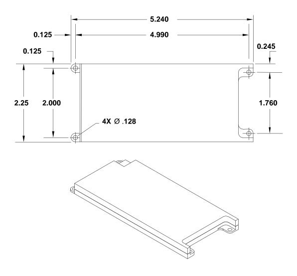
Figure 1. – Hole Mounting
