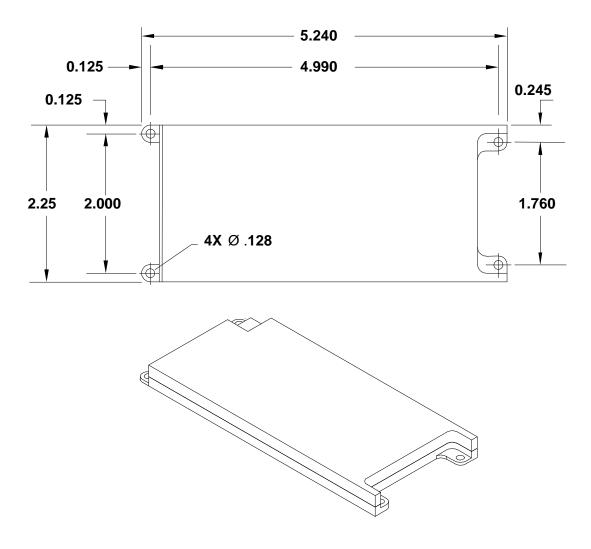
Figure 1. – Hole Mounting
