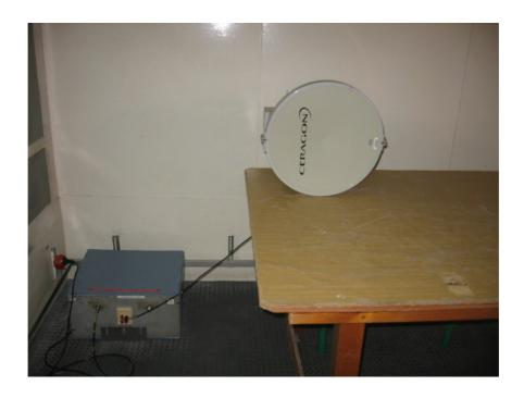
Photograph No.6 Setup for conducted emission measurements at the AC power lines
