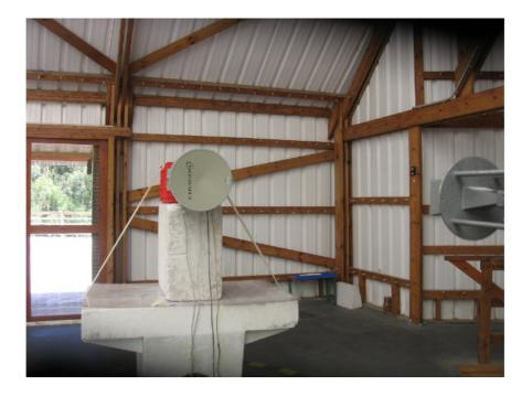
Photograph No.5 Setup for spurious emission field strength measurements at the OATS above 40 GHz range
