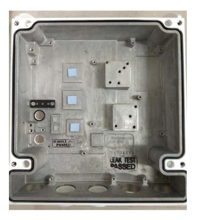
Photograph No.10 "FibeAir IP-20C 24" internal view with main board removed
