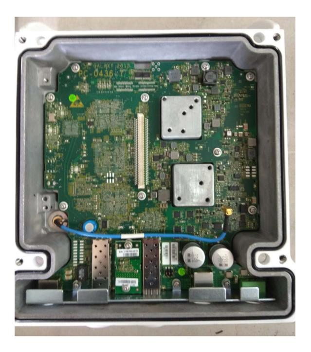
Photograph No.3 "FibeAir IP-20C 24" internal view without Tx/Rx module
