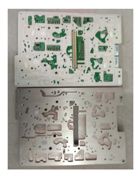
Photograph No.9 RF module PCB and shielding compartment, second side view
