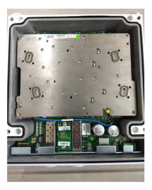
Photograph No.2 "FibeAir IP-20C 24" internal view without diplexer
