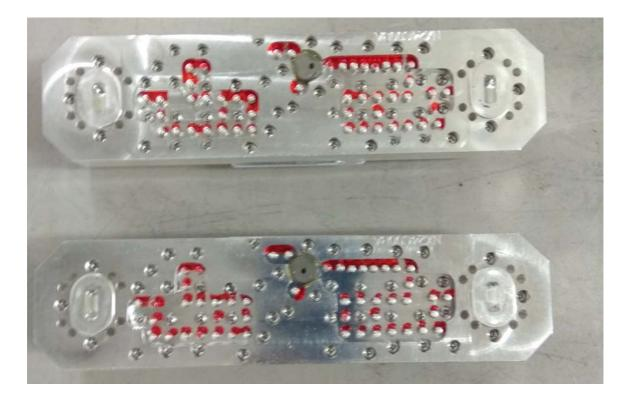
Photograph No.12 "FibeAir IP-20C 24" diplexer second side view
