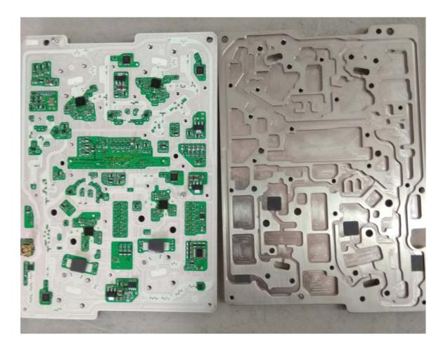
Photograph No.8 RF module PCB and shielding compartment, front view
