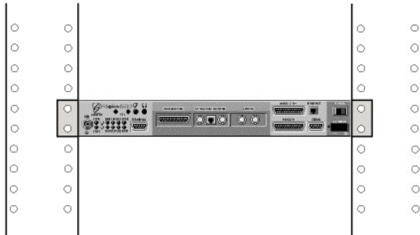
Figure 3-2 Rack Mount Assembly
