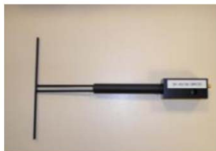
Figure 1 – Satimo COMOSAR Validation Dipole
