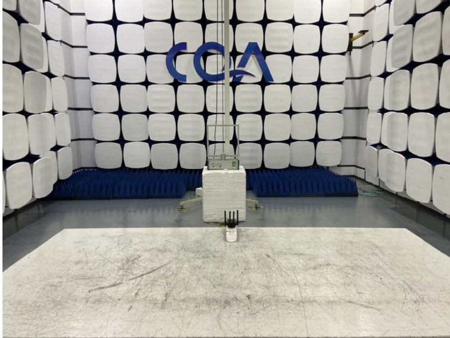
Radiated spurious emission Test Setup-1(Below 30MHz)
