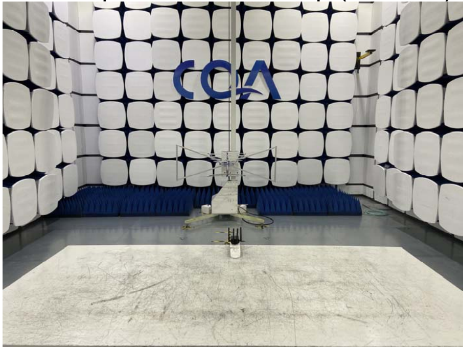
Radiated spurious emission Test Setup-2(30MHz-1GHz)
