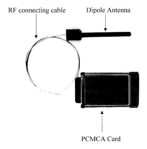
The PCMCIA card body and the Dipole Antenna are connected by a piece of RG-178 RF cable. There is not any connector or replaceable part use in the assembly.
