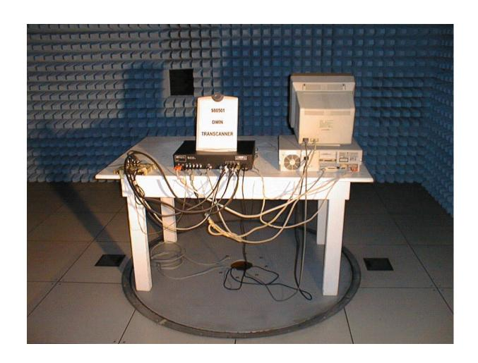
Radiated emission test (Rear view)
