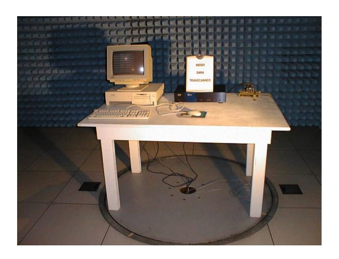
Radiated emission test (Front view)
