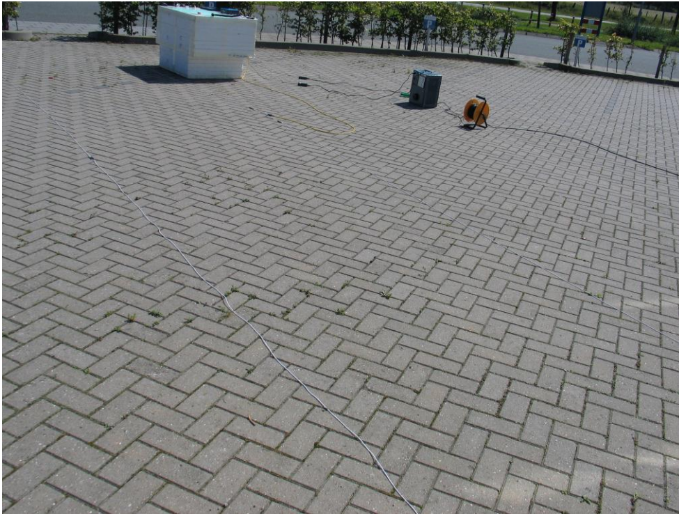
EUT in combination with 12m loop antenna
