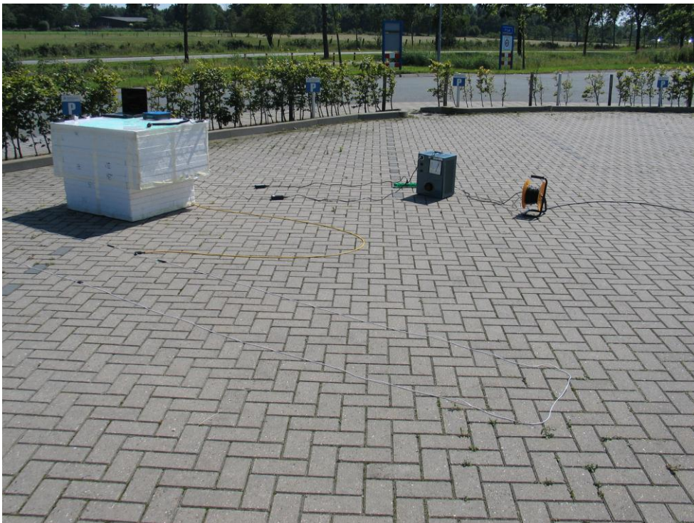
EUT in combination with 6m loop antenna
