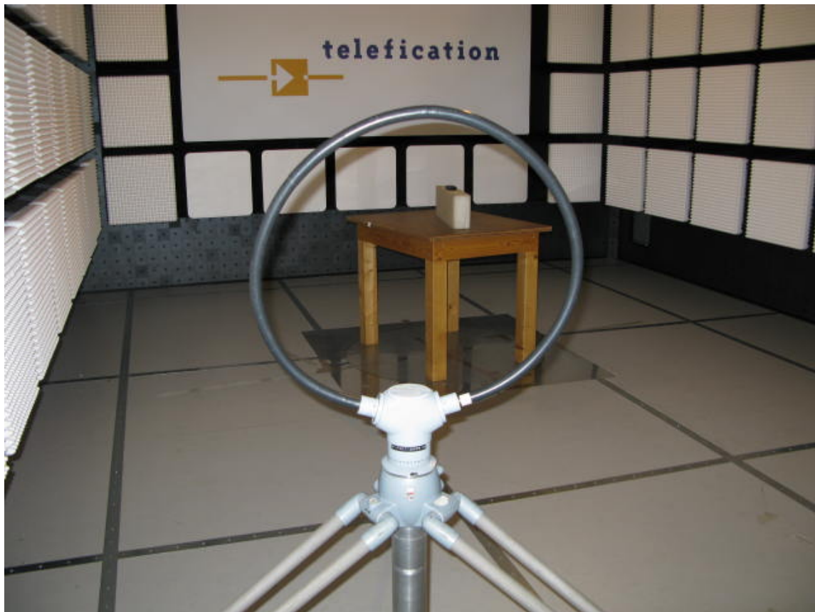
Photograph 2: Test setup field strength measurements (< 30 MHz)
