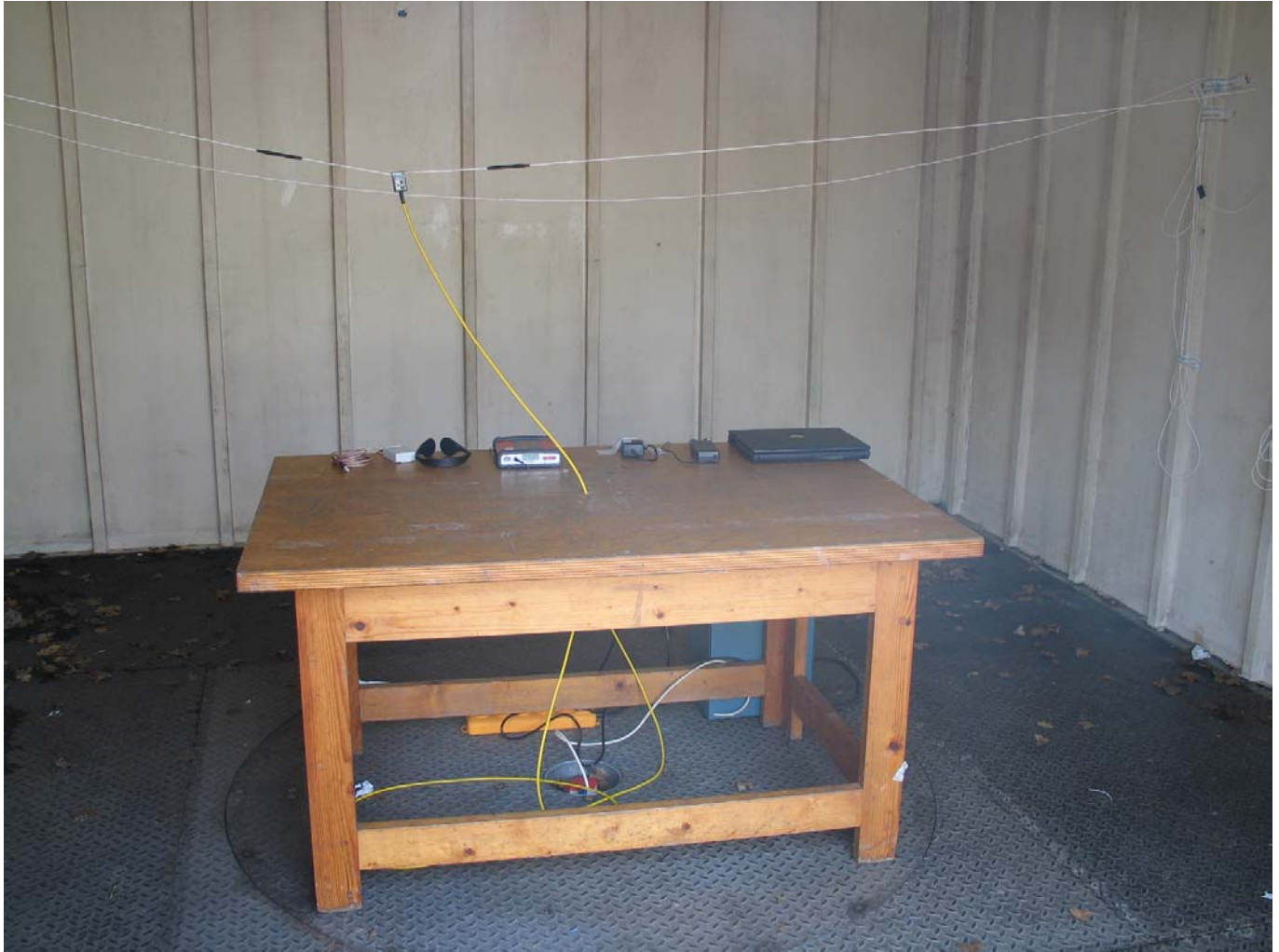
Photo 2: Radiated Emission measurement set up, front view
