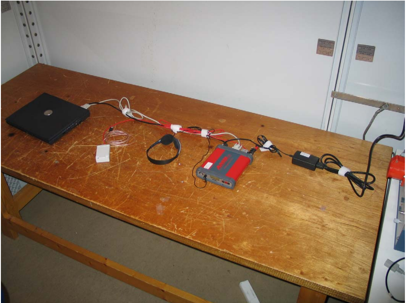
Photo 4: Conducted Emission measurement set up
