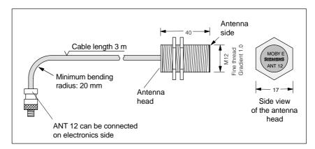
Figure 5-35 Dimensioned drawing of the ANT 12
