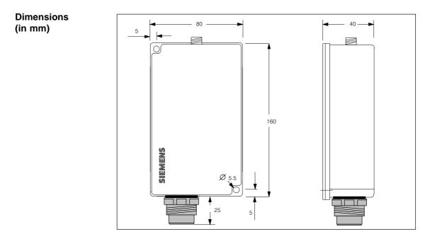
Figure 5-33 Dimensioned drawing of SLG 75
