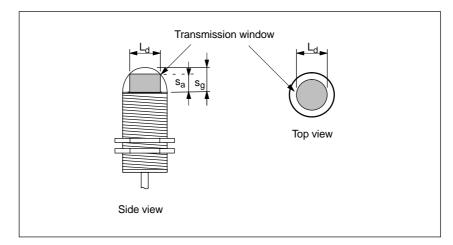
Figure 5-22 Transmission window of the ANT12
