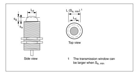
Figure 5-23 Transmission window of the ANT18
