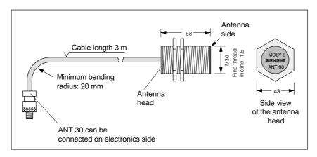
Figure 5-37 Dimensioned drawing of the ANT 30
