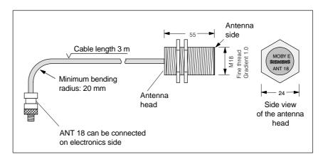
Figure 5-36 Dimensioned drawing of the ANT 18
