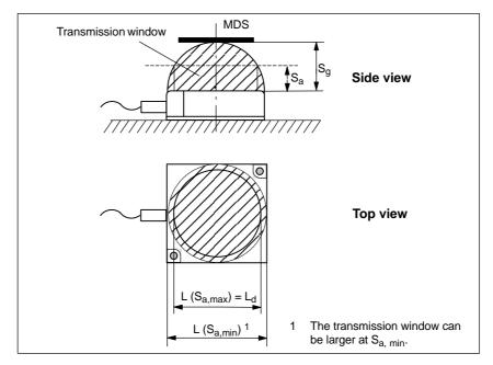
Figure 5-21 Transmission window of the ANT 1
