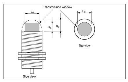
Figure 5-24 Transmission window of the ANT 30
