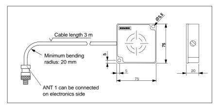
Figure 5-34 Dimensioned drawing of the ANT 1
