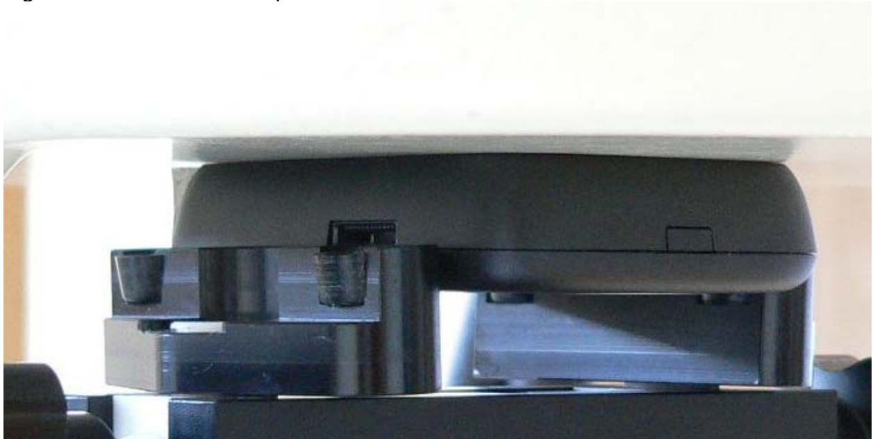
Fig. 13: Body worn configuration Siemens Ay, PCS 1900 without accessory, displays towards the phantom, gap= 0mm.
