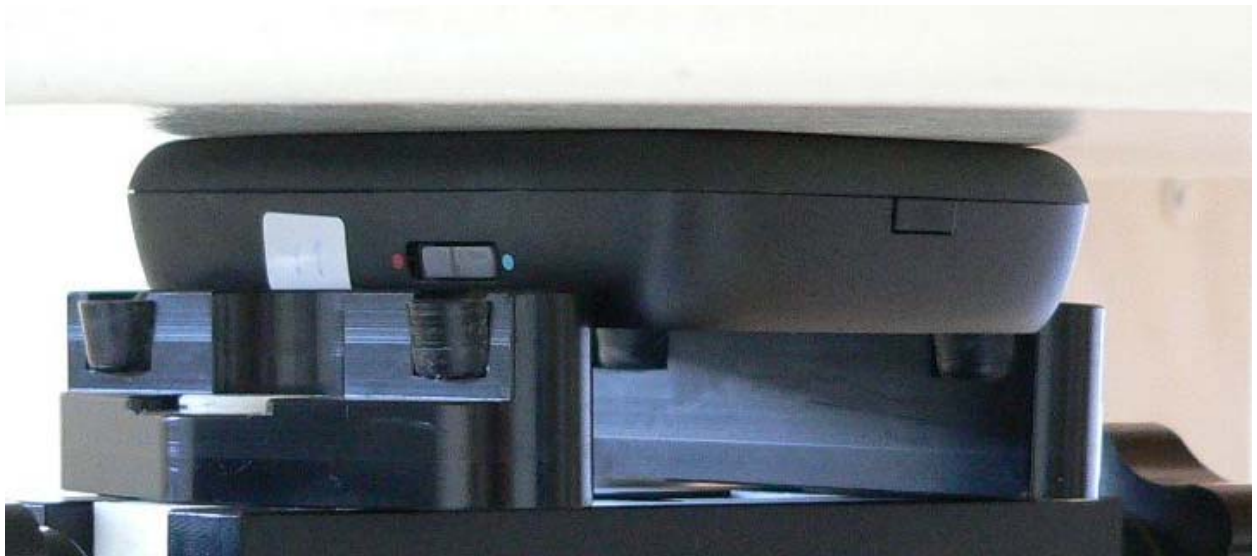
Fig. 14: Body worn configuration Siemens Ay, PCS 1900, without accessory, display towards the ground, gap= 0 mm.
