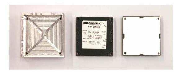
DC-DC converter – located on reverse side of digital board
