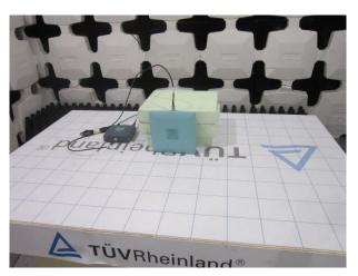
RADIATED TEST SETUP
