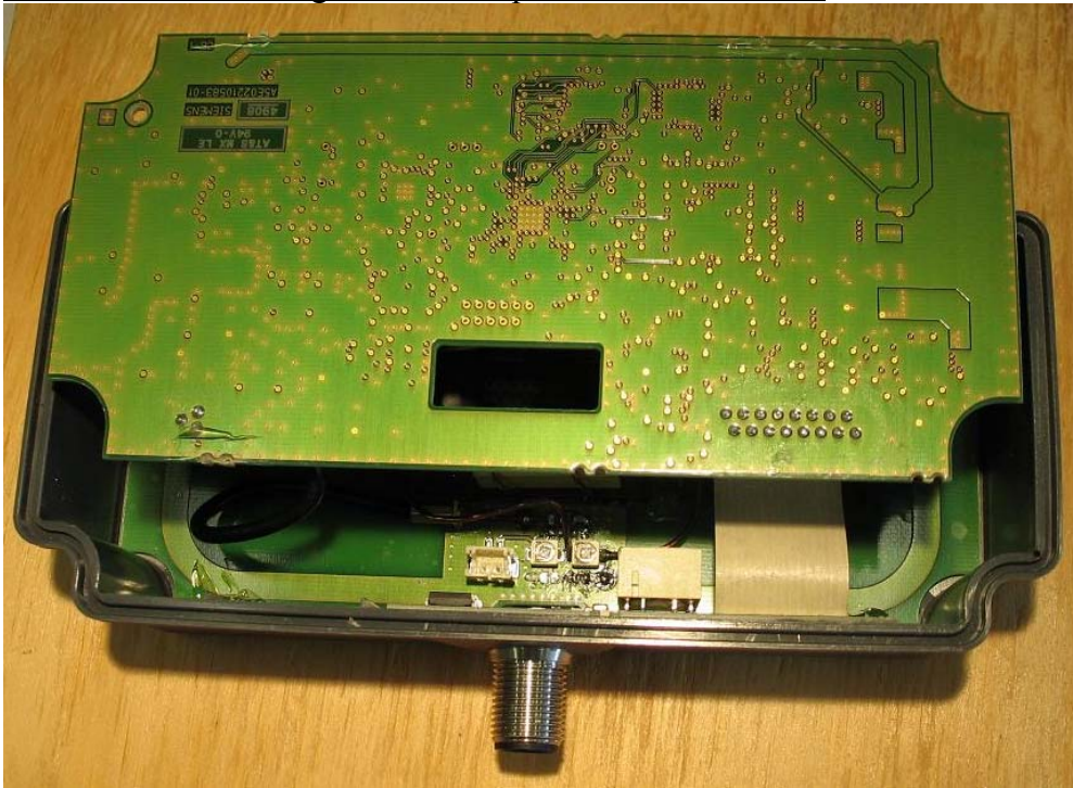
RF382R in it's housing – two PCBs placed over each other
