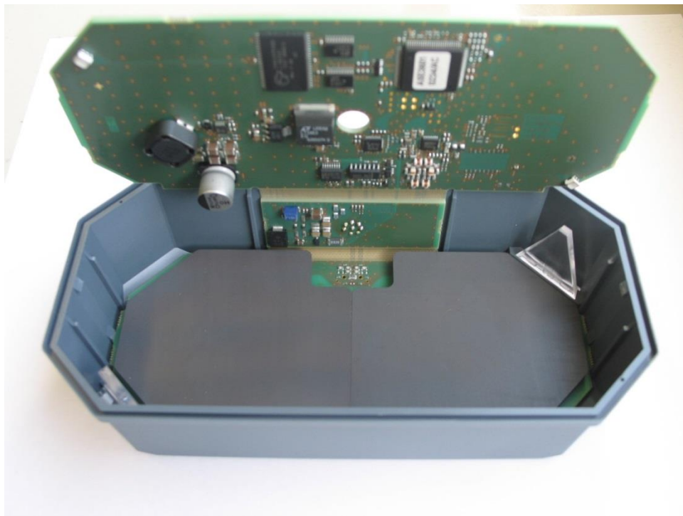
Fig. 4: PCB fixed in housing with ferrite
