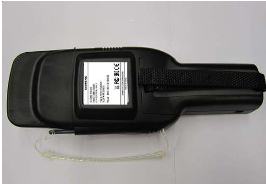
Picture 5. Simatic RF350M outside label location.
