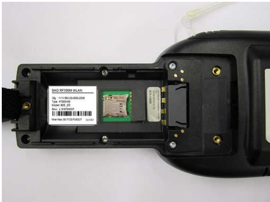
Picture 6. Simatic RF350M inside label location.
