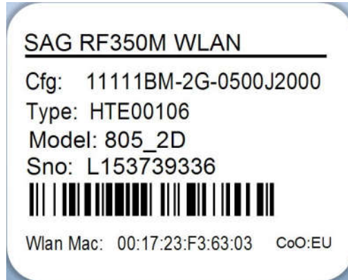
Picture 3. Simatic RF350M inside label.
