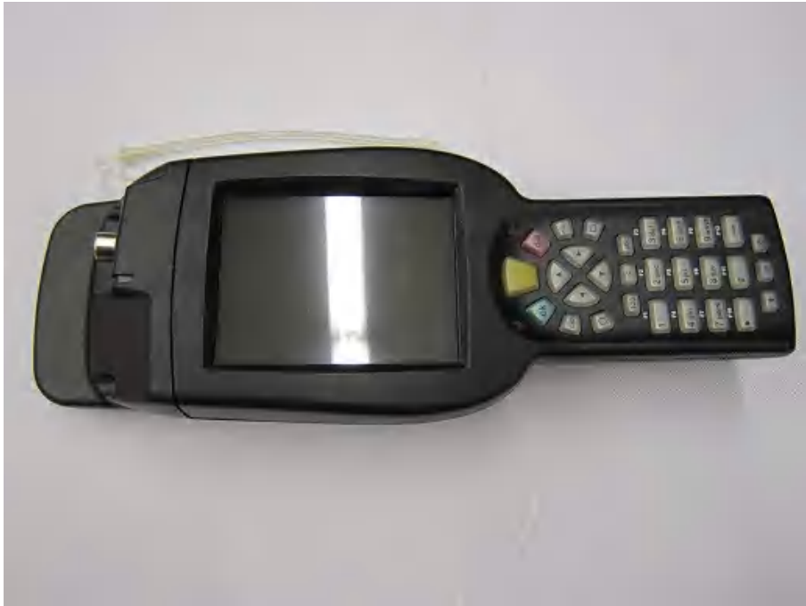
Picture 7. Simatic RF350M with an external antenna connector front side.
