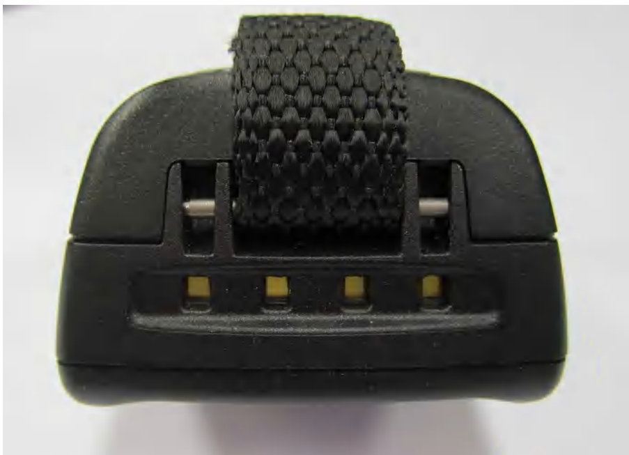
Picture 6. Simatic RF350M bottom side.
