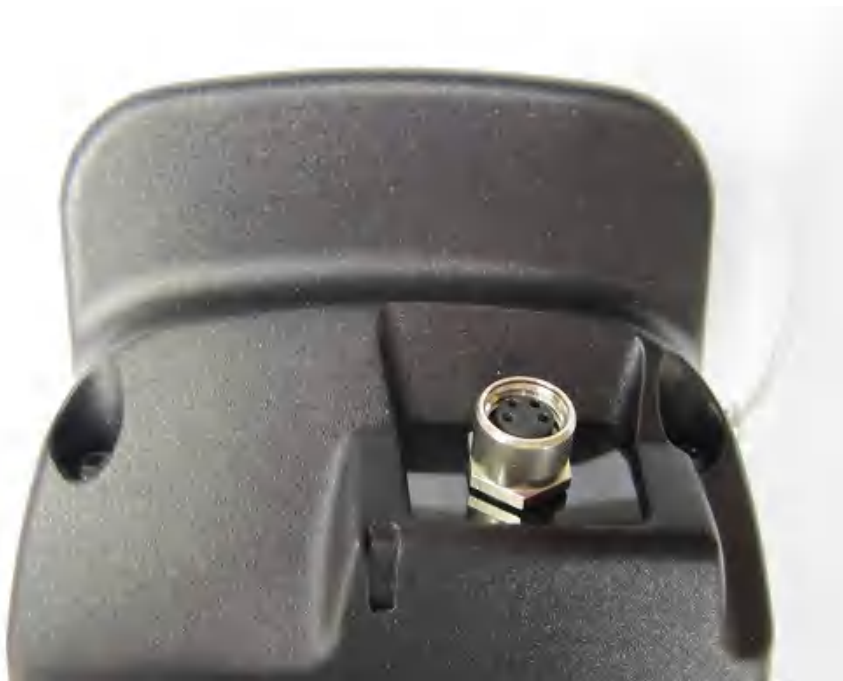
Picture 8. Simatic RF350M with an external antenna connector top side.
