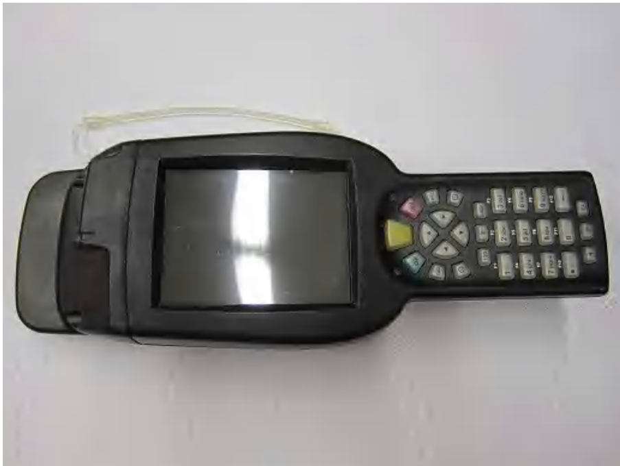
Picture 1. Simatic RF350M front side.
