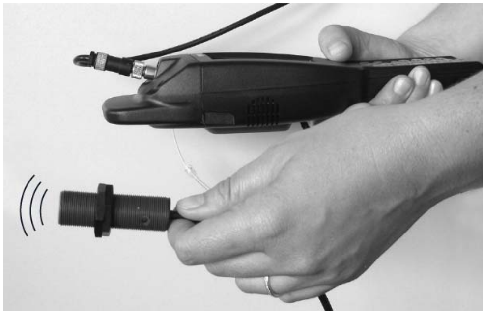
Figure 3-4 Propagation of the RF field with external antenna
