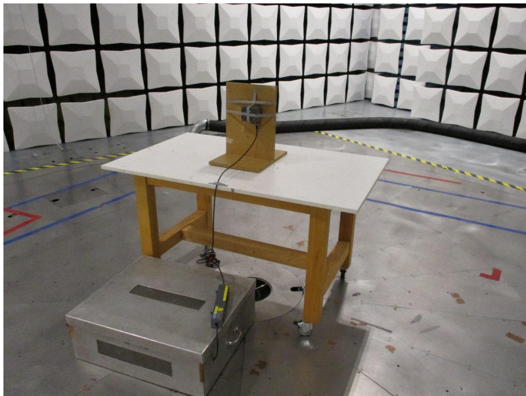
Radiated Emission Measurement (Alternate Test Site)
