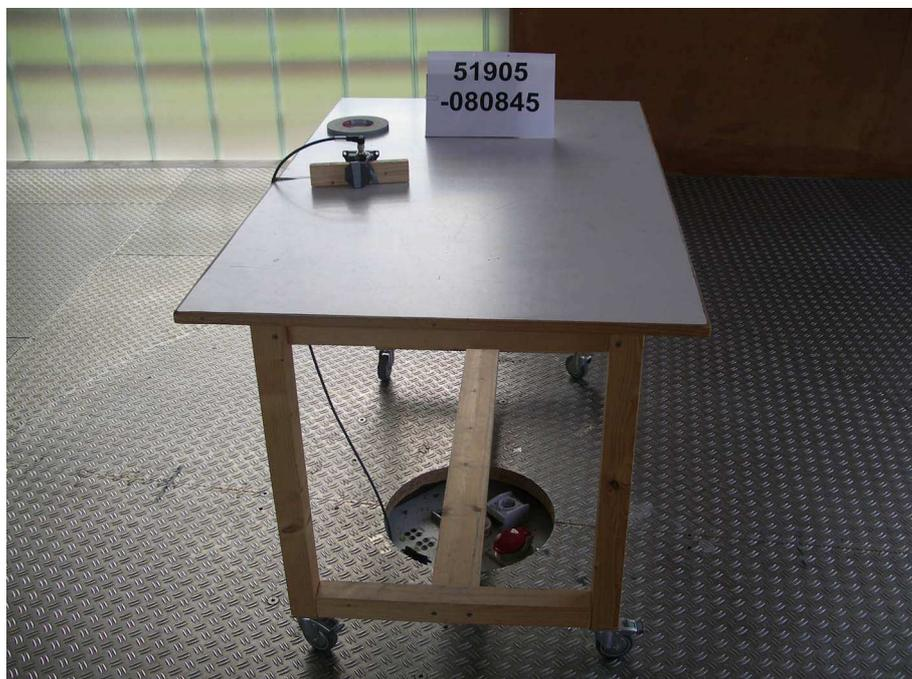
**Test setup for radiated emission measurement
