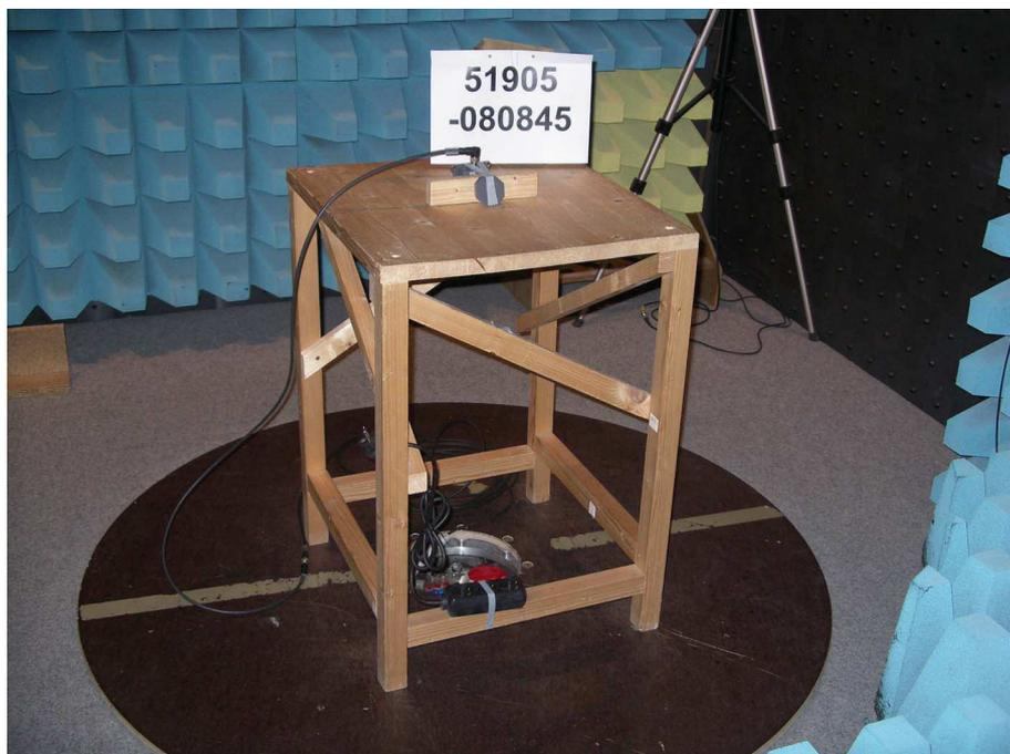
**Test setup for radiated emission measurement
