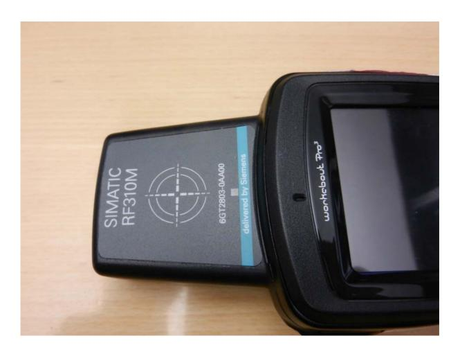
SIMATIC RF310M with new Handheld unit (Workabout Pro<sup>3</sup>
