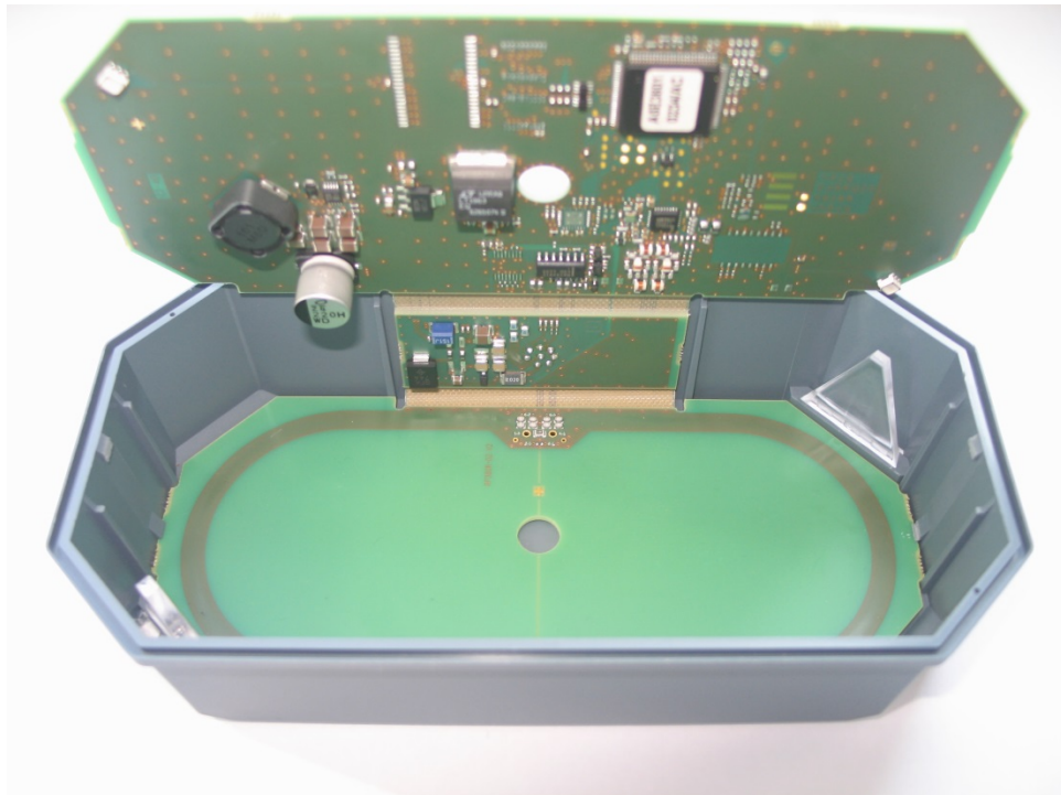
Fig. 4: PCB fixed in housing
