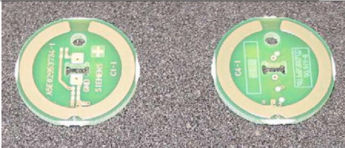
RF220R-IO-Link antenna PCB (front and back side)
