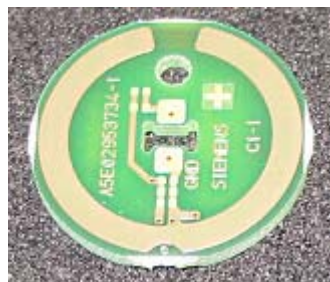
RF220R antenna PCB; front and backside
