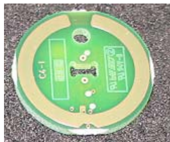
RF220R antenna PCB; front and backside
