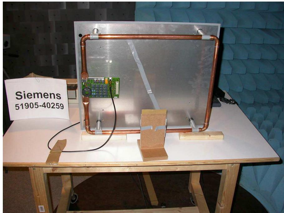
**Test setup for radiated emission measurement
