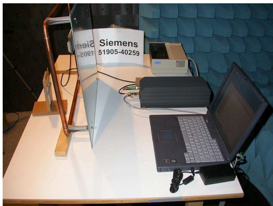
**Test setup for radiated emission measurement
