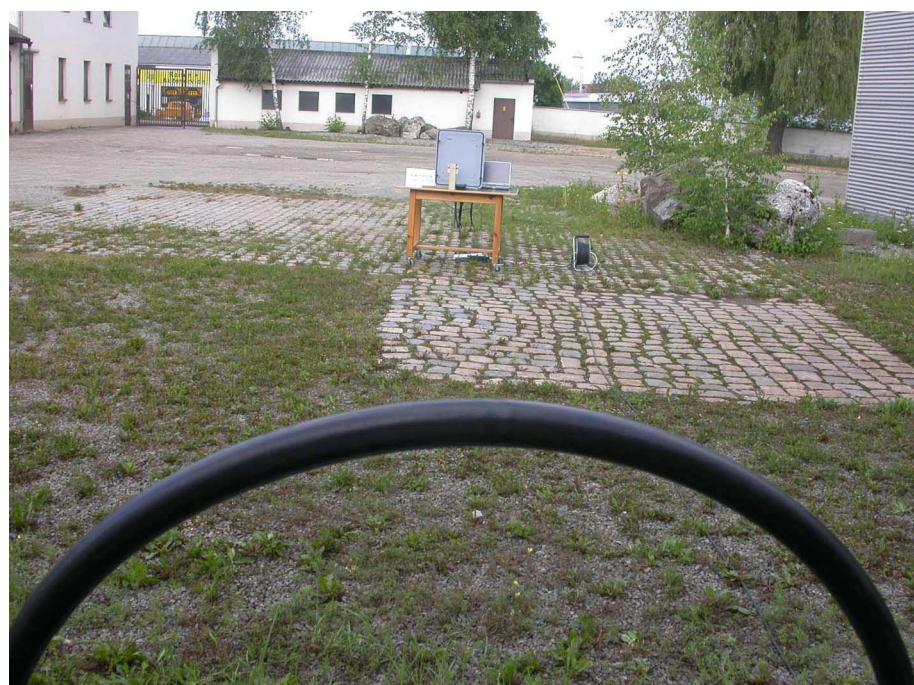
**Test setup for radiated emission measurement
