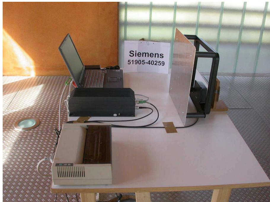
**Test setup for radiated emission measurement
