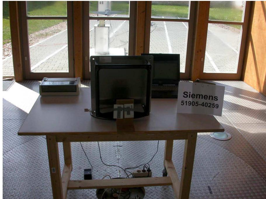
**Test setup for radiated emission measurement
