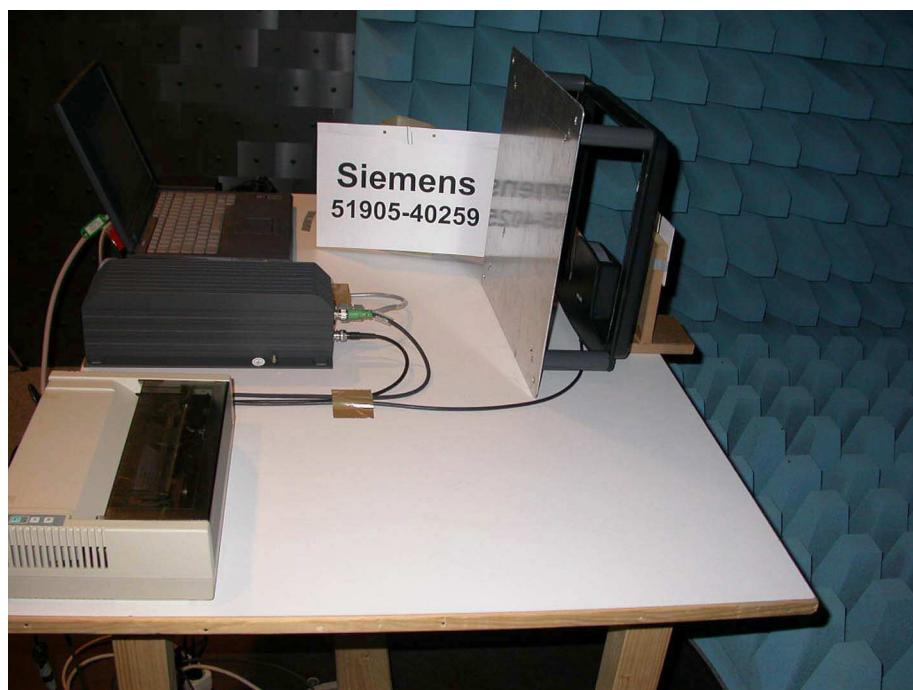
**Test setup for radiated emission measurement
