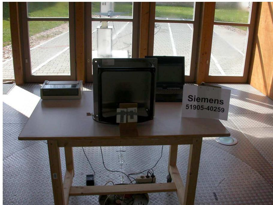
**Test setup for radiated emission measurement
