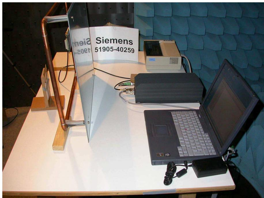
**Test setup for radiated emission measurement
