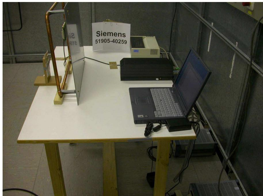
**Test setup for spurious radiation measurement**
