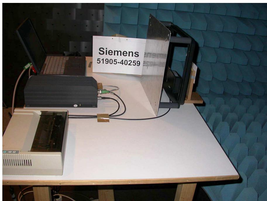
**Test setup for radiated emission measurement
