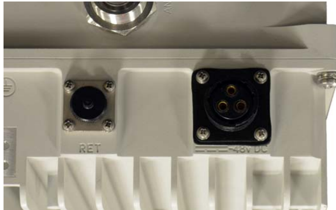
Figure 3-4 iRM4451 RET and -48v DC (power) connectors location
