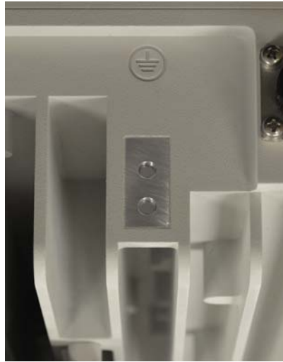
Figure 3-6 iRM4451 ground connector location
