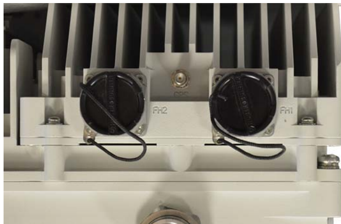
Figure 3-5 iRM4451 GPS and fronthaul connectors location
