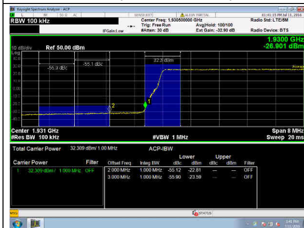
10 MHz 64QAM (bottom channel)
