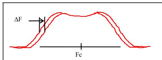
The technique for measuring a wave form with an index of modulation greater than (1) involves a process of observing the wave form on the spectrum analyzer and measuring the time difference at the slope of the wave form (  $\Delta F = 1 / \Delta t$ ).
