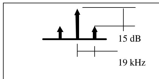
The technique for measuring a wave form with an index of modulation less than (1) involves a different process for observing the wave form. The equation used to calculate the side band modulation is as follows:
