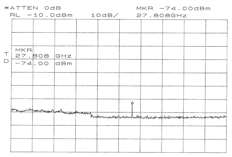
START 25.000GHz STOP 30.000GHz \*RBW 100kHz VBW 100kHz \*SWP 10.0sec
