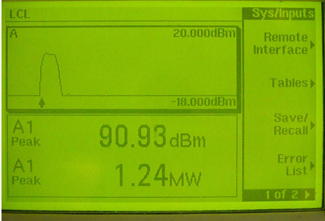
#33: 1.6µs RF Pulse with RF Pulse Shaping
