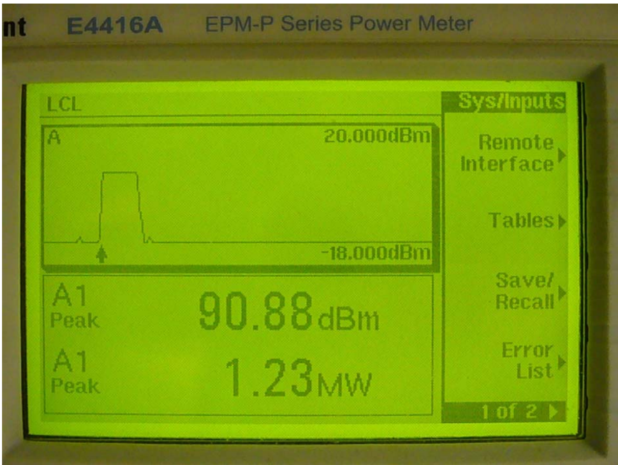
Plot #32: 1.6µs RF Pulse with NO RF Pulse Shaping
