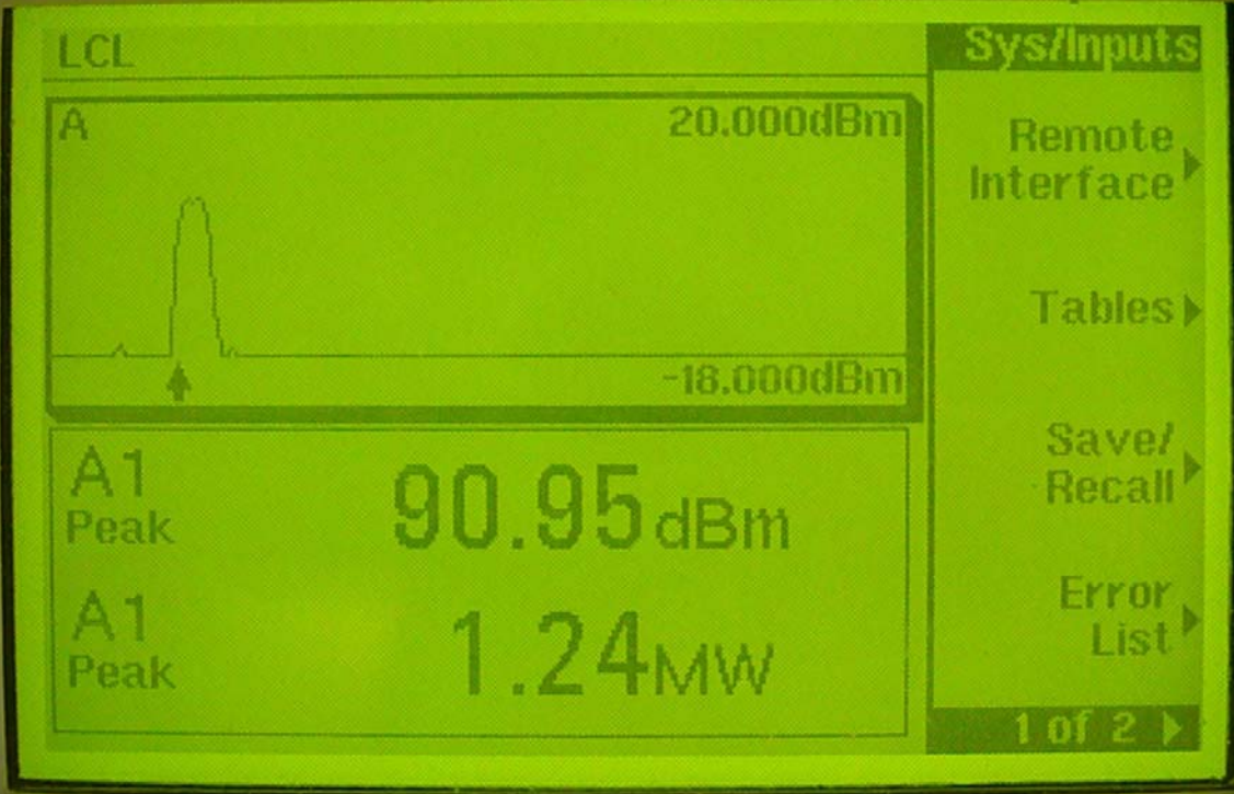
Plot #31: .8μs RF Pulse with RF Pulse Shaping
