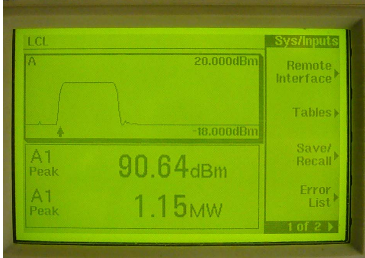
Plot #29: 4.5μsRF Pulse with RF Pulse Shaping
