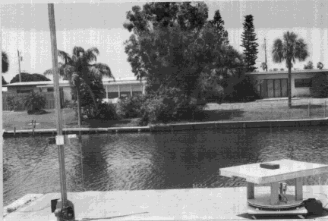
Figure G. Orientation of the EUT and pickup antenna at the 3 meter open field test site. Highest emissions were obtained with a vertically polarized dipole antenna. The highest emissions were 1.4dB below the specification limit at a frequency of 88.9MHz.
