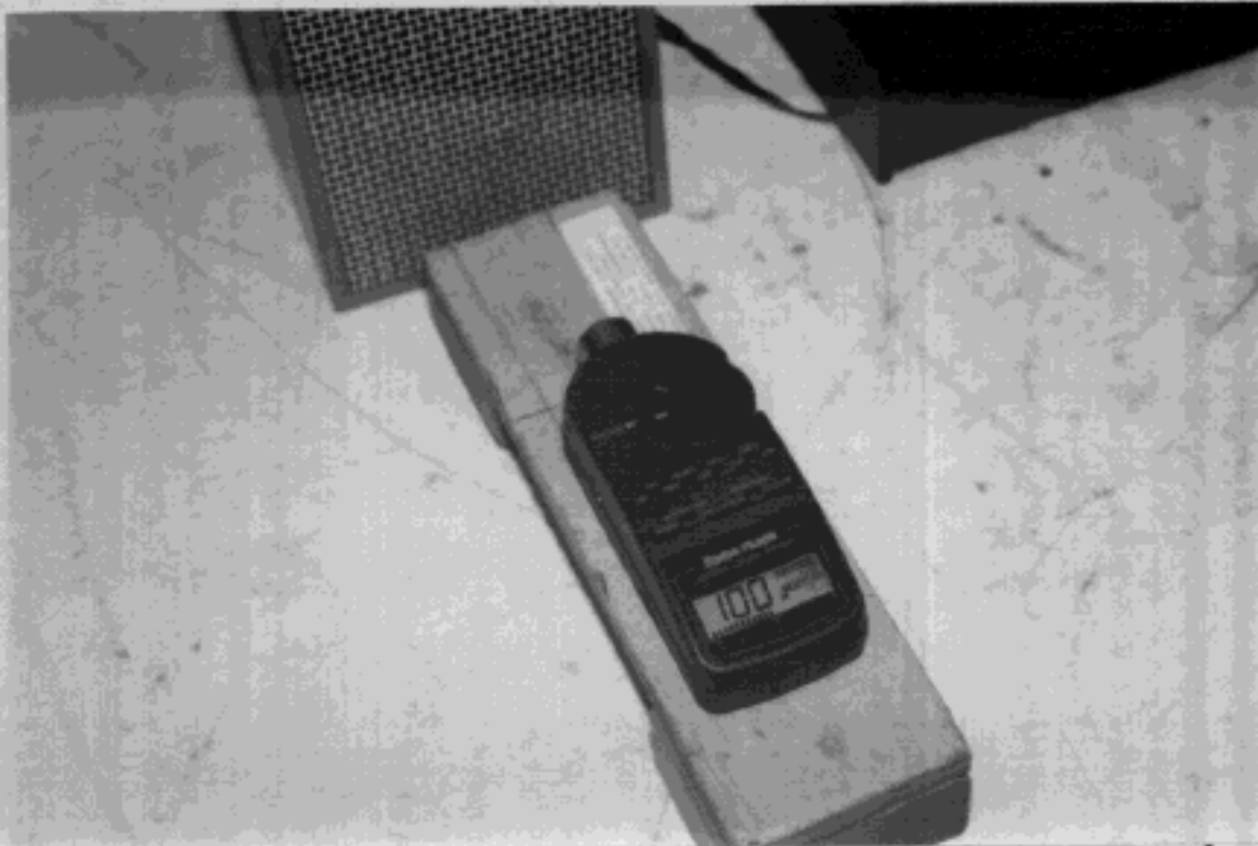
Figure C. Setup for determining the required 100dB sound pressure level. Digital audiometer at right. 4 inch speaker housed in a sealed wood enclosure on left. Spacing is 10 cm.
