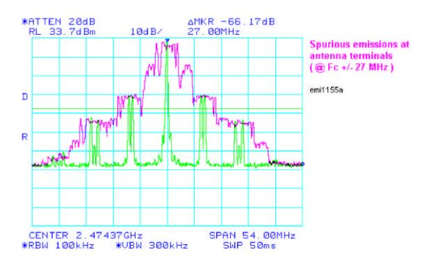
Plot illustrating compliance to 47CFR 90.210(b)(2) and 74.637(a)(2) at 100 to 150 % of the Authorized bandwidth:
