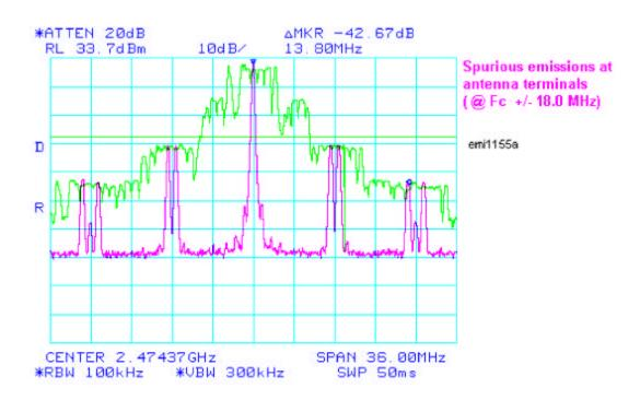
Plot illustrating compliance to 47CFR 90.210(b)(1) and 74.637(a)(1) at 50 to 100 % of the Authorized bandwidth:
