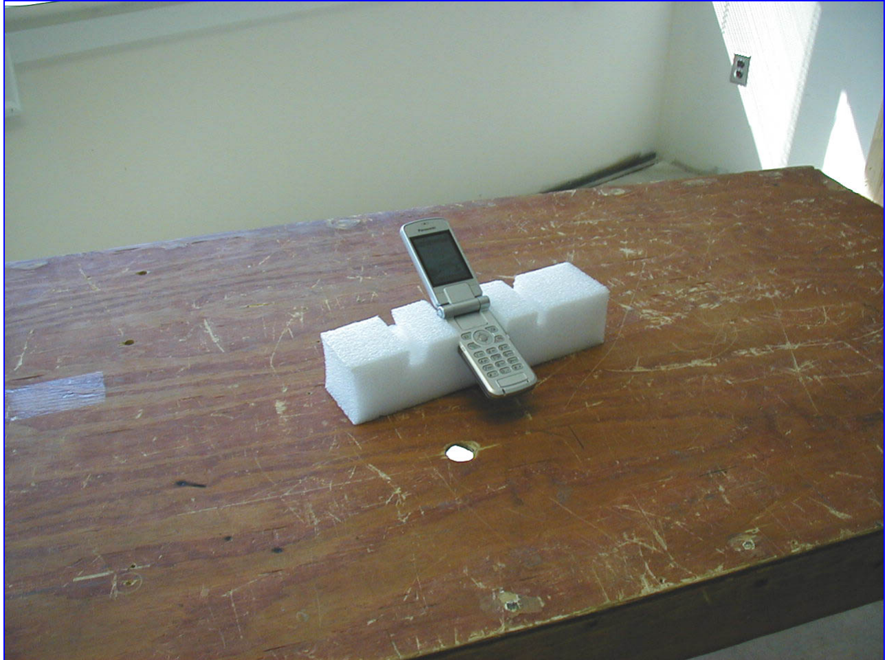
Photograph 2 EIRP measurement Setup
