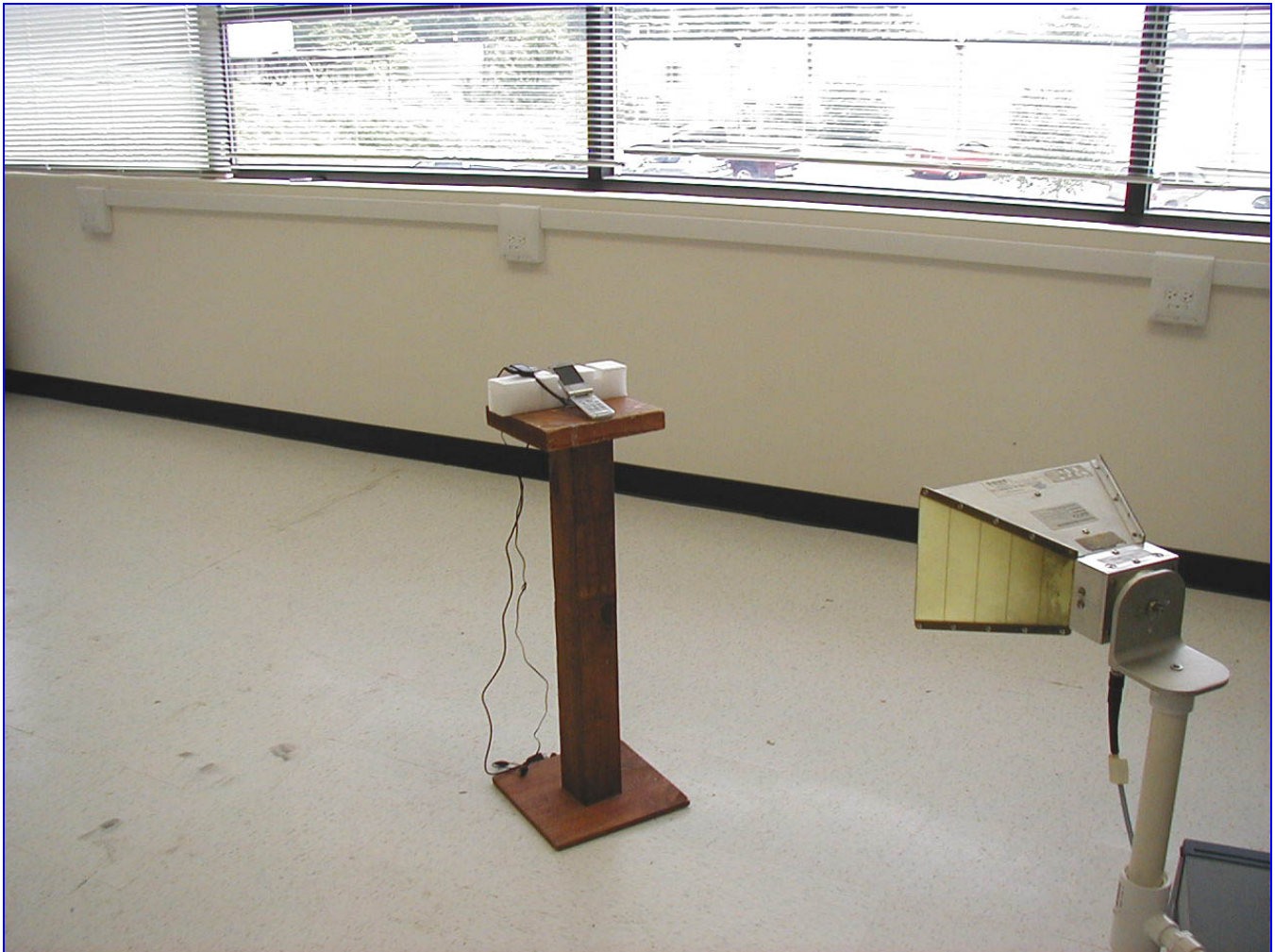
Photograph 6 Radiated emissions measurement Setup
