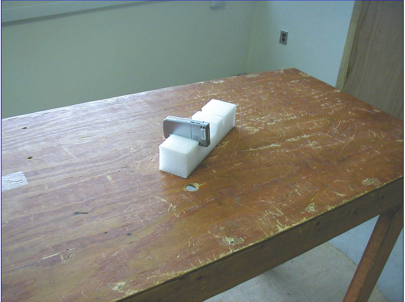
Photograph 4 EIRP measurement Setup
