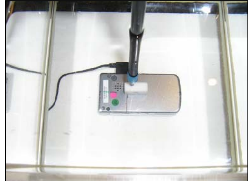
Figure 22: Positional photograph of the Panasonic EB-VS3 Handset Rear Facing 15mm from Phantom with SHF.
