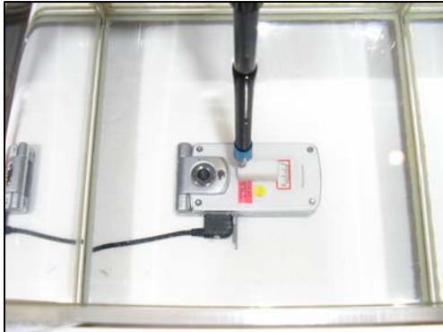
Figure 21: Positional photograph of the Panasonic EB-VS3 Handset Front Facing 15mm from Phantom with SHF.
