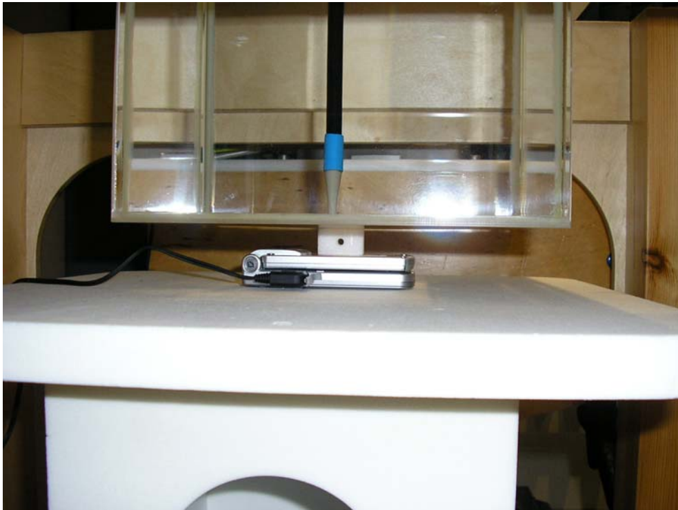
Figure 25: Positional photograph of the Panasonic EB-VS3 Handset 15mm from Phantom with SHF.
