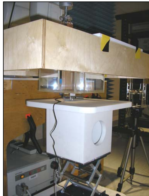
Figure 24: Positional photograph of the Panasonic EB-VS3 Handset Rear Facing 15mm from Phantom with SHF
