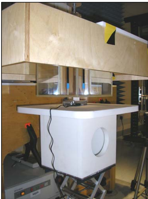
Figure 23: Positional photograph of the Panasonic EB-VS3 Handset Front Facing 15mm from Phantom with SHF
