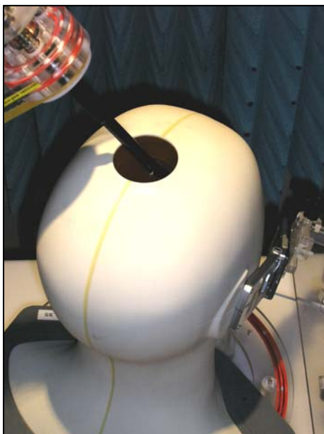
Figure 19: Positional photograph of the Panasonic EB-VS3 Handset in the Right-hand Cheek Position
