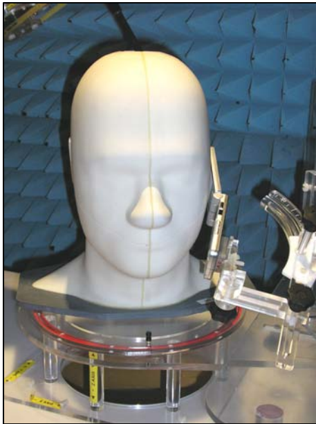
Figure 17: Positional photograph of the Panasonic EB-VS3 Handset in the left-hand Cheek Position
