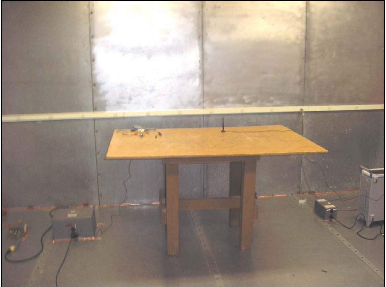
Photograph 1. Conducted Emissions, Test Setup
