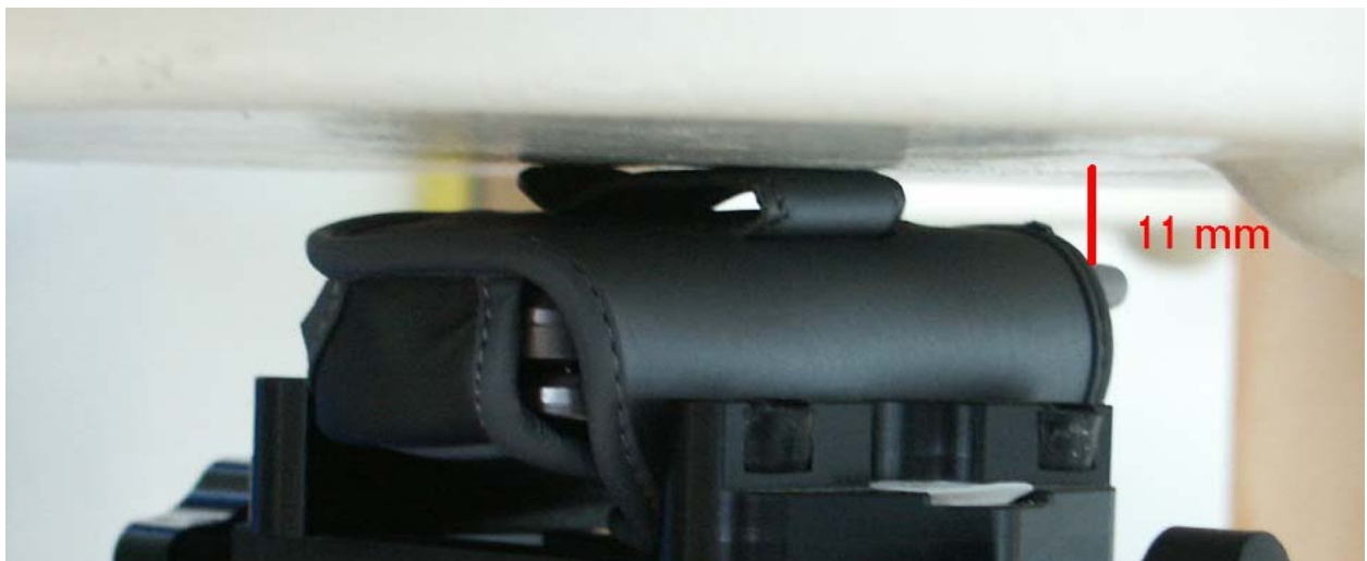
Fig. 29: Body worn configuration, carry case without headset (1 TX slot). Also used for the repeated measurement with activated Bluetooth
