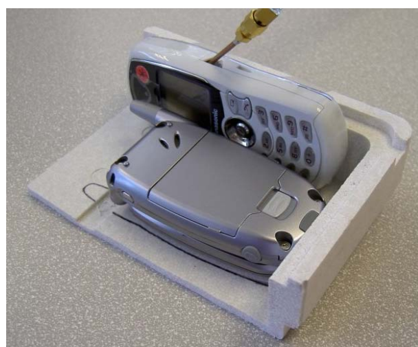
Fig. 9: Provided coupler to control the output power, position for PCS 1900.
