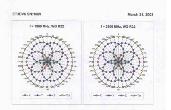
Isotropy Error ( $\phi$ ),  $\theta = 0^{\circ}$
