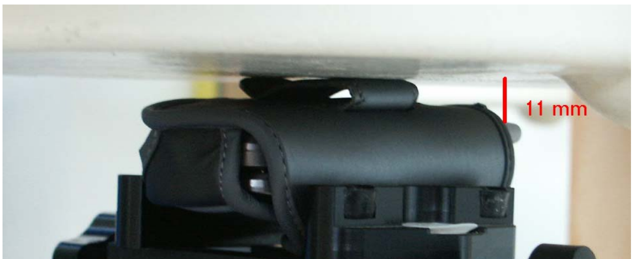
Fig. 24: Body worn configuration, carry case without headset (1 TX slot).
