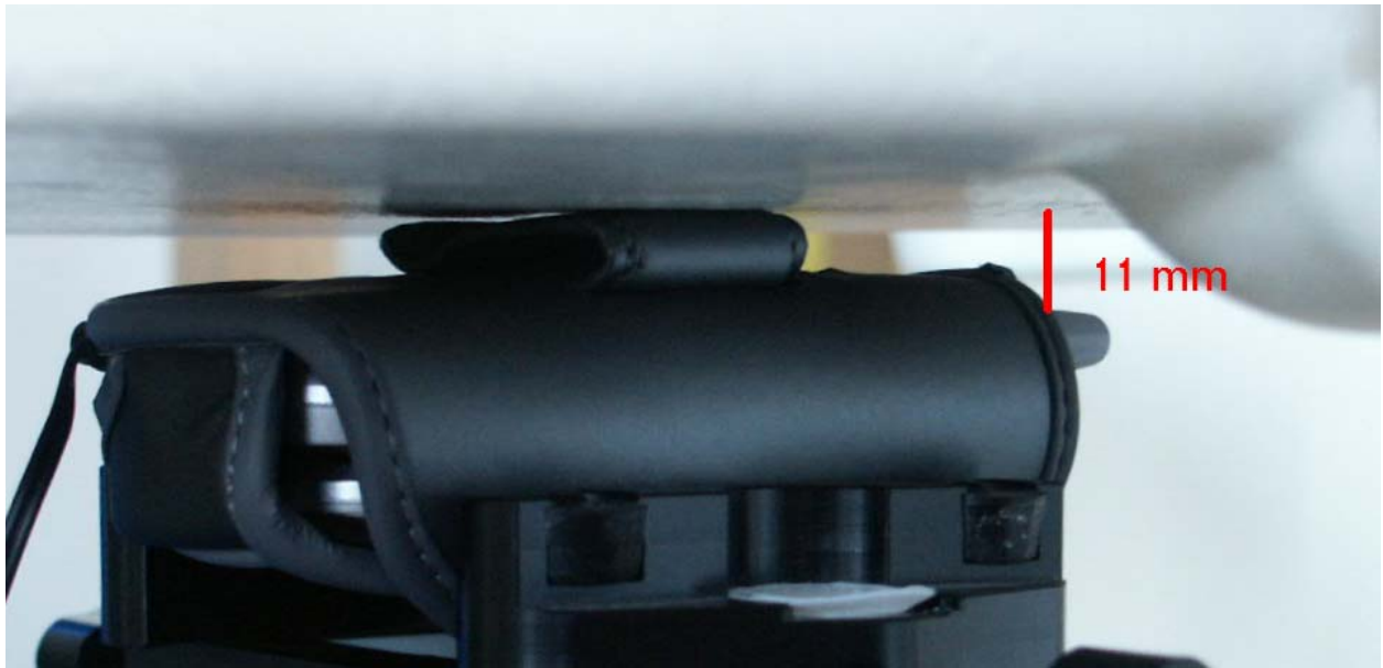
Fig. 23: Body worn configuration, carry case with headset (1 TX slot). Also used for the repeated measurement with activated Bluetooth.
