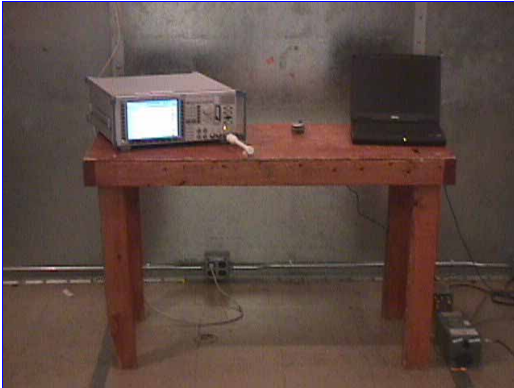
Photograph 1. Conducted Limits, Test Setup
