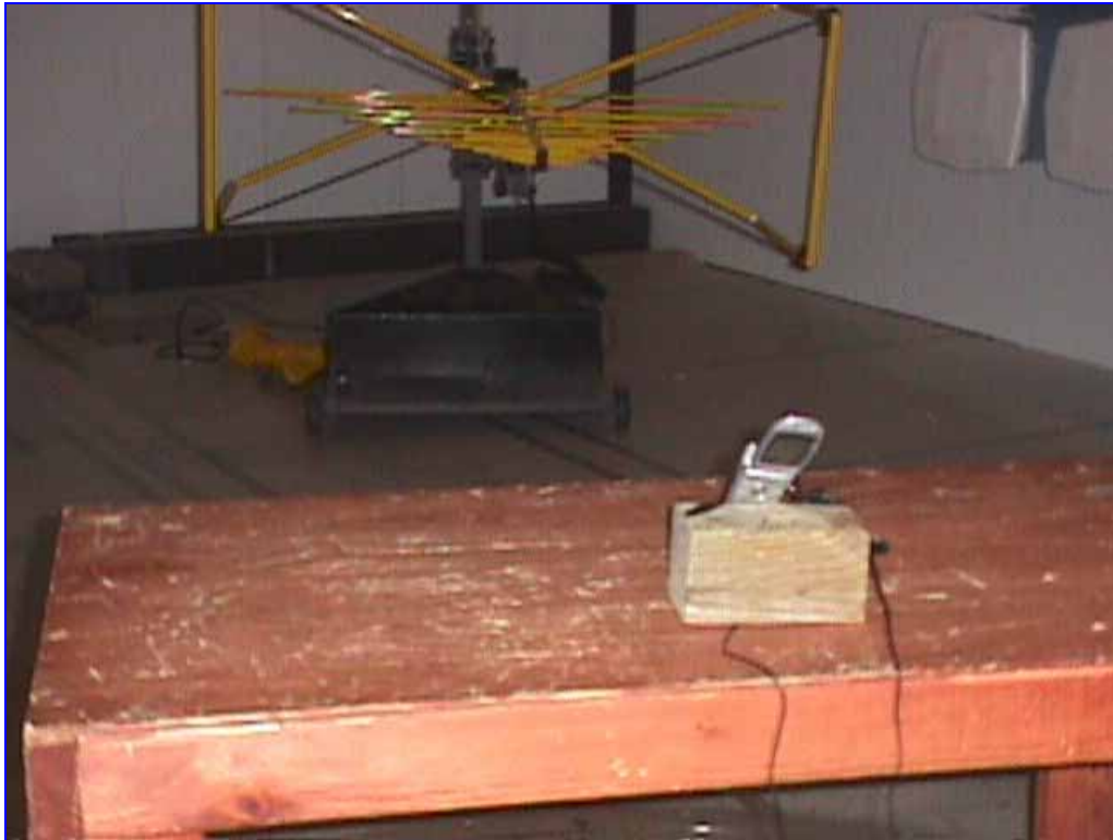
Photograph 2. Intentional Radiated Emission Limits, Test Setup
