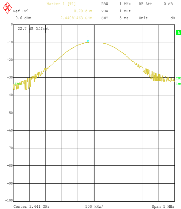
Title: 70944JD07 Panasonic EUT:X800 FCC Part 15.247 Comment A: Peak Output Power Middle Channel Input Voltage 93.5V Date: 17.DEC.2004 16:23:49
