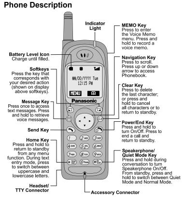
You can enter up to 32 characters by pressing the number keys. The keypad is also used to enter text as described in "Text Entry Operations", Chapter 4
