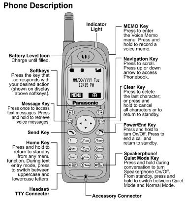
You can enter up to 32 characters by pressing the number keys. The keypad is also used to enter text as described in *"Text Entry Operations"*, *Chapter 4*.
